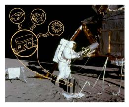
Figure: A thermoelectric generator directly converts heat into electricity with no moving parts. The long term reliability of these systems has encouraged NASA to use thermoelectric generators in many space probes since the 1960s (up to 35 years unattended). Today, thermoelectrics are being considered for terrestrial applications such as automotive and industrial waste heat recovery as well as solar-electricity generation.
