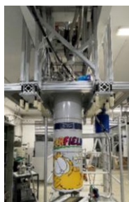
Fig. 1 We have two top-loading Triton 400 systems. The rear system has a 14 T magnet with cancellation coil. The front system has a 91 mm bore size 12 T magnet. The loading and measurement are performed in the up-floor room. We designed a special mounting structure for the front system. Two steel beams are anchored at the building framework, to which the dilution fridge is hung with 16 20-mm steel rods (inside the vertical aluminum profiles). The fridge has a clear surrounding and the structure and the load bearing is over 3,000 kg.
